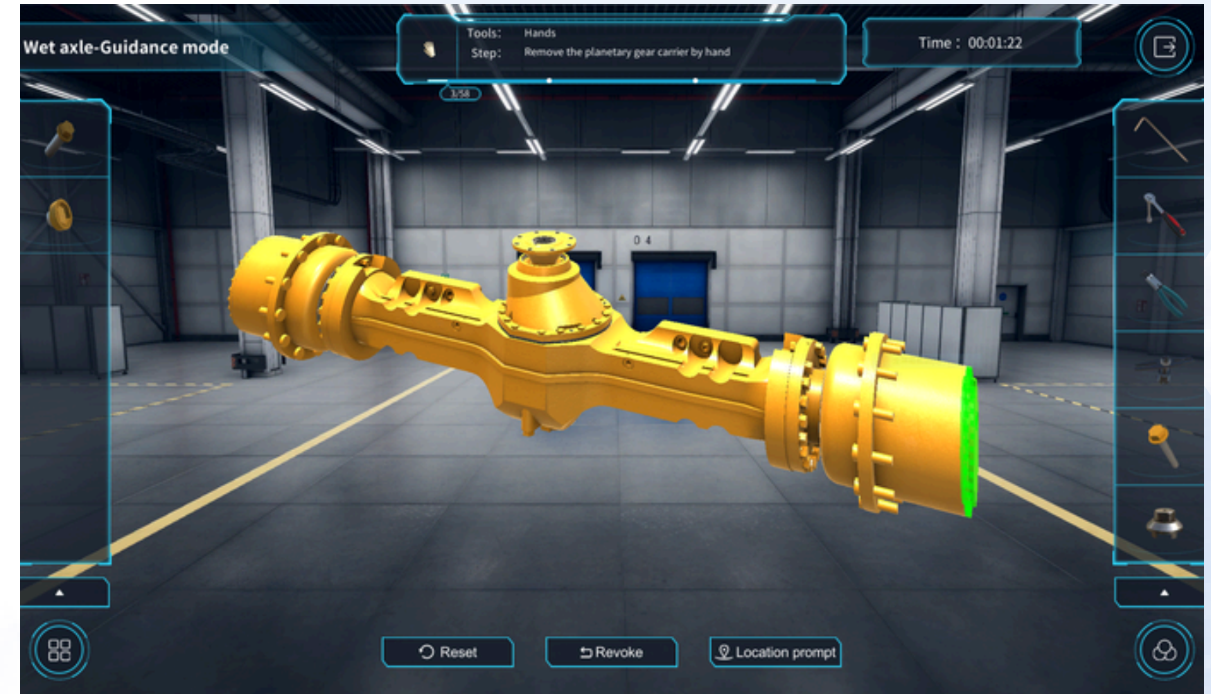
Interactive training exercises on wet axle disassembly, dry axle disassembly, and manual transmission disassembly
