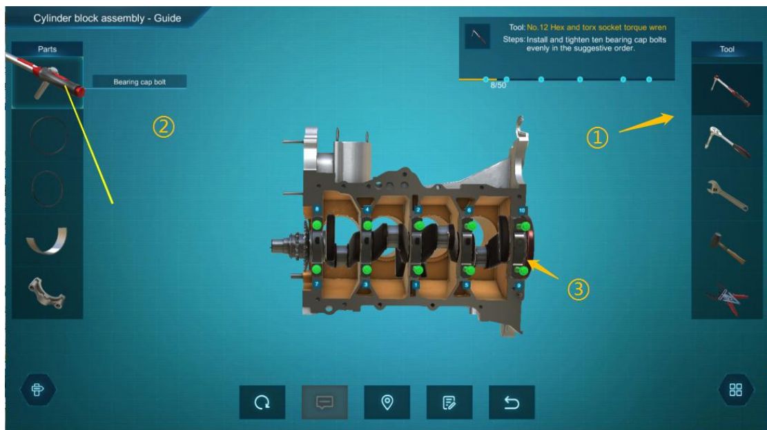
Figure 4-2-3-4b Operating instructions on installing a bolt/nut
