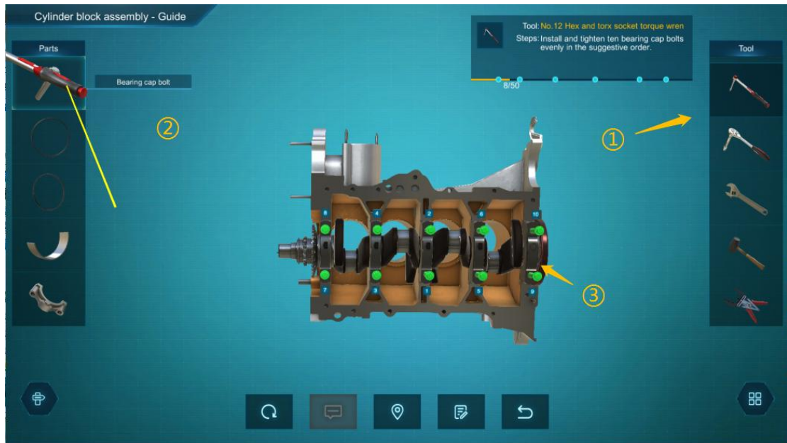
Figure 4-2-3-4c Operating instructions on installing lubricating parts
