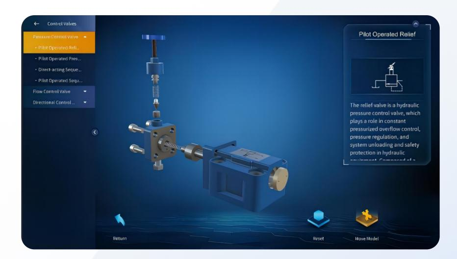
It clearly displays the internal structure of a pilot-operated relief valve, which consists of a pilot valve and a main valve.
