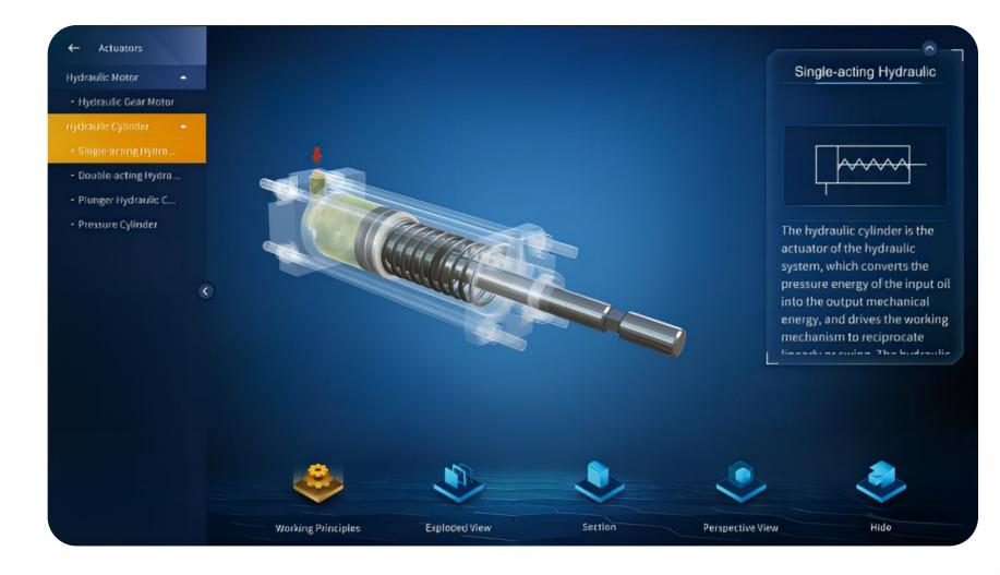
It demonstrates the process of converting pressure energy into mechanical energy through the use of a single-acting hydraulic cylinder, employing 3D animation effects.
