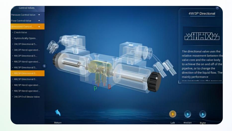
It creates a virtual scene to demonstrate the process of how the directional valve utilizes the relative movement between the valve core and the valve body to change the direction of the liquid flow.
