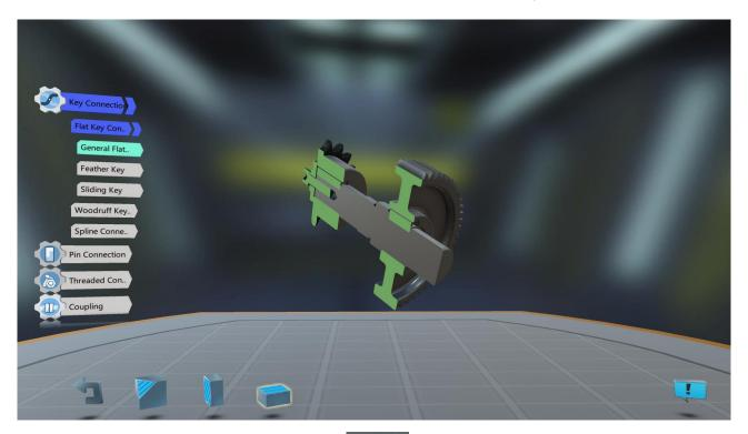
4.2.9 Click the Arbitrary Section button. A cutting plane occurs to help section a component arbitrarily. Put the dissecting plane through the object from any angle first. Then press the right stylus button to dissect the object. Cast the stylus ray on any dissected part and press the middle button to move it. Press the left button to restore the dissected object.
